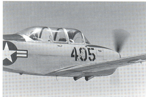
The ideal sight picture for a wingman has the aileron-flap junction on the trailing edge of the wing lined up with the last cowl latch, indicating a 45° angle-off from the lead aircraft. Both top and bottom of the wing are visible, indicating proper step-down. (Lou Drendel)
